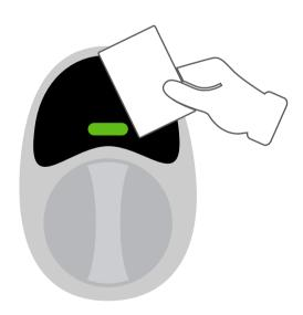
...or by touching your smart card or fob to the large black button and turning the lock's handle when the light turns green.
