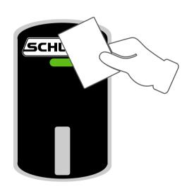
...or by touching your card or fob to the lock and turning its handle when the light turns green.
