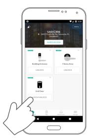
While in front of the lock, you can unlock it by either tapping "LOCK/UNLOCK" on the unit dashboard and turning the lock' handle when prompted by the mobile app...
